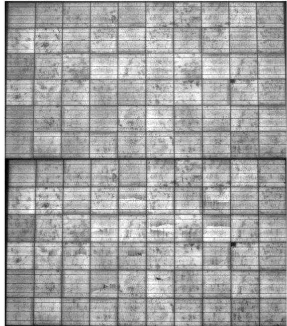
**Figure 10:** EL image of panel with 160 $\mu$ m cells (III run) before test sequence (top) and after shaker and TC200 (bottom).
