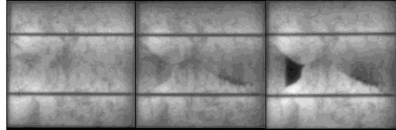
**Figure 3:** EL image of a cell initial (left) after shaker (middle) and after TC400 (right). Clearly visible is the origin and evolution of cracks because of mechanical and further growth due to thermal stress.
