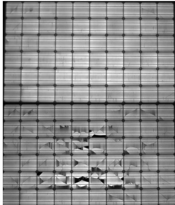
**Figure 6:** Panel EL image before (top) and after (bottom) mechanical load test before optimization of the mono crystalline cells.
