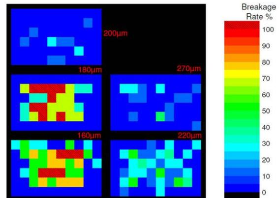
**Figure 4:** Average spatially resolved breakage rate for 60 cells panels made from cells with varying thicknesses after shaker test.
