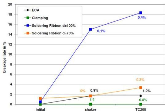
**Figure 12:** Breakage rate of two panels soldered with different ribbon thicknesses (blue and orange) and two panels made with non soldering techniques - mechanical clamping (green) and ECA (black). Above the data points is noted the relative power degradation.
