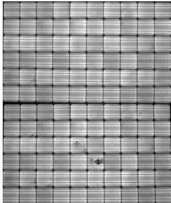
**Figure 7:** Panel EL image before (top) and after (bottom) mechanical load test of the optimized mono cells.
