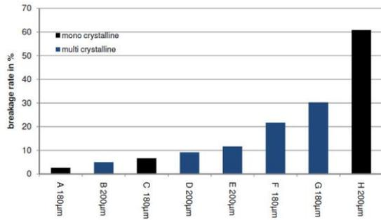
**Figure 11:** Mono and multi crystalline cell supplier comparison in breakage rate after shaker test.
