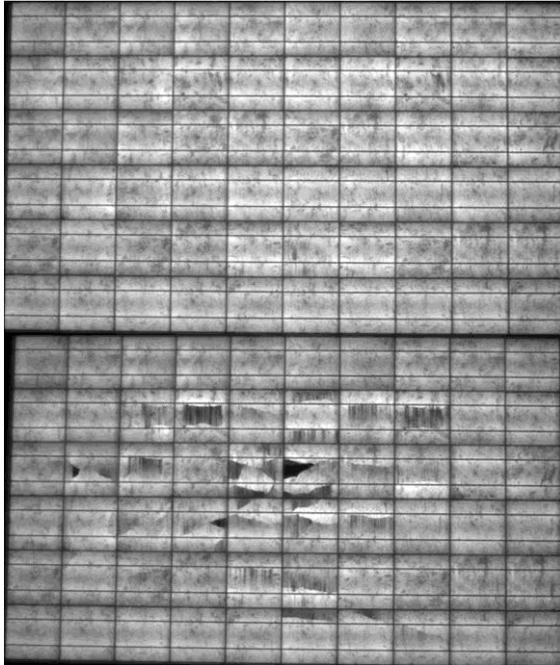
**Figure 8:** EL image of panel with 160 $\mu$ m cells (II run) before test sequence (top) and after shaker and TC400 (bottom).
