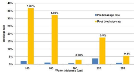
**Figure 5:** Average breakage rate depending on wafer thickness before and after shaker test. Values for power degradation are also noted.
