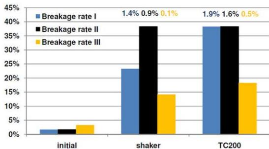
**Figure 9:** Shaker test and thermal cycling test of panels with 160 $\mu$ m cells. Cells were mechanically optimized from round I to II and again before III.
