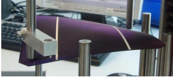
**Figure 1:** Twist tester setup.
